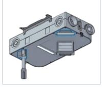
Removable filter holder, 45° oriented to optimize pressure drop in every unit's configuration
